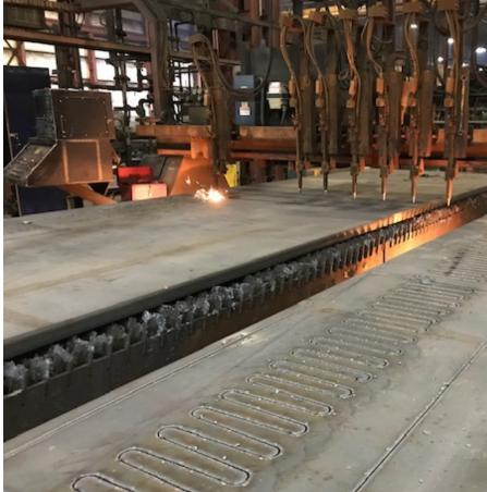
When compared to water-jet, oxyfuel presents a more optimal method for finger joints--and it's due to more than just the cost of the process.
